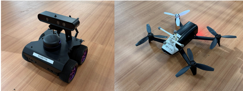
Figure 5-2. Husarion Rosbot 2 Pro (left) and Parrot Bebop 2.0 (right). At least 4 motion capture markers are attached to each robot for tracking.
